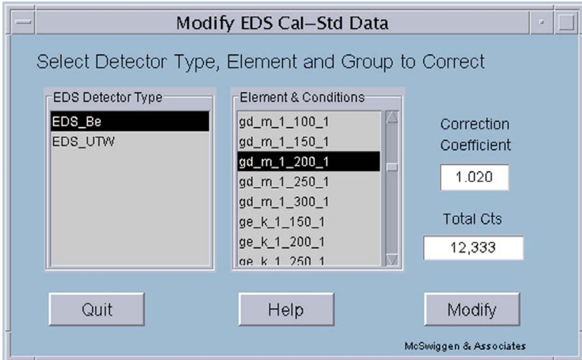
When *EDS\_Cal-Std\_mod* runs it displays two data sets, one for EDS detectors with ultra-thin windows (EDS\_UTW), and the other for EDS detectors with Be windows (EDS\_Be). Select the appropriate one for your system. Now select the element and desired operating conditions that you would like to modify. Most of the elements have been standardized at 10, 15, 20, 25 and 30 kV.
